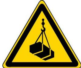
Suspended loads are dangerous. Working beneath a suspended load is prohibited. There is a risk of fatal injury. Safety and accident prevention guidelines applicable for forklift, stacker
