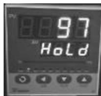
In Hold state, press the
